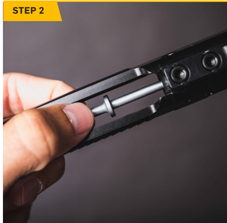
Slide the firing pin out through the rear of the carrier.
