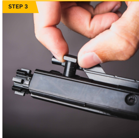
Rotate the cam pin to the side so that it is clear of the gas key. Lift the cam pin out of the bolt carrier group.
