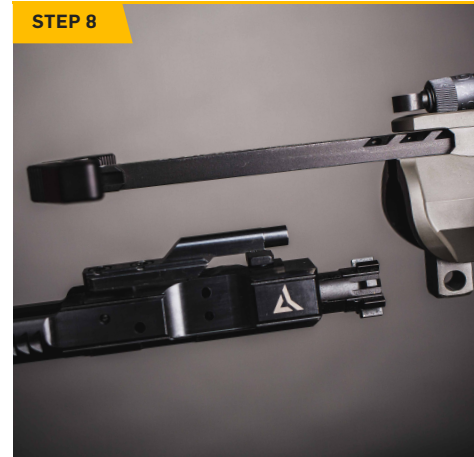
Remove the bolt carrier group from the upper receiver.
