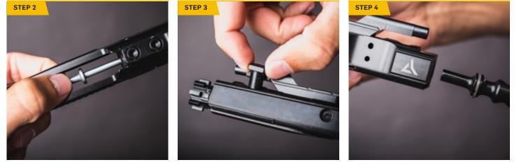
Slide the firing pin out through the rear of the carrier.
