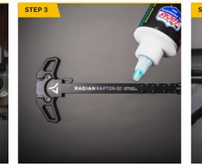
Place lubricant on the sides and top of the charging handle. Lubricate the takedown pins.
