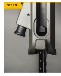
Pull the charging handle fully towards the rear. Remove the charging handle by moving it so that the expanded end of the charging handle passes through the cut-out in the guide track of the upper receiver.
